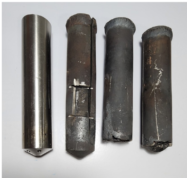
Figure 12. Examples of clogged burners due to severe coke formation.
