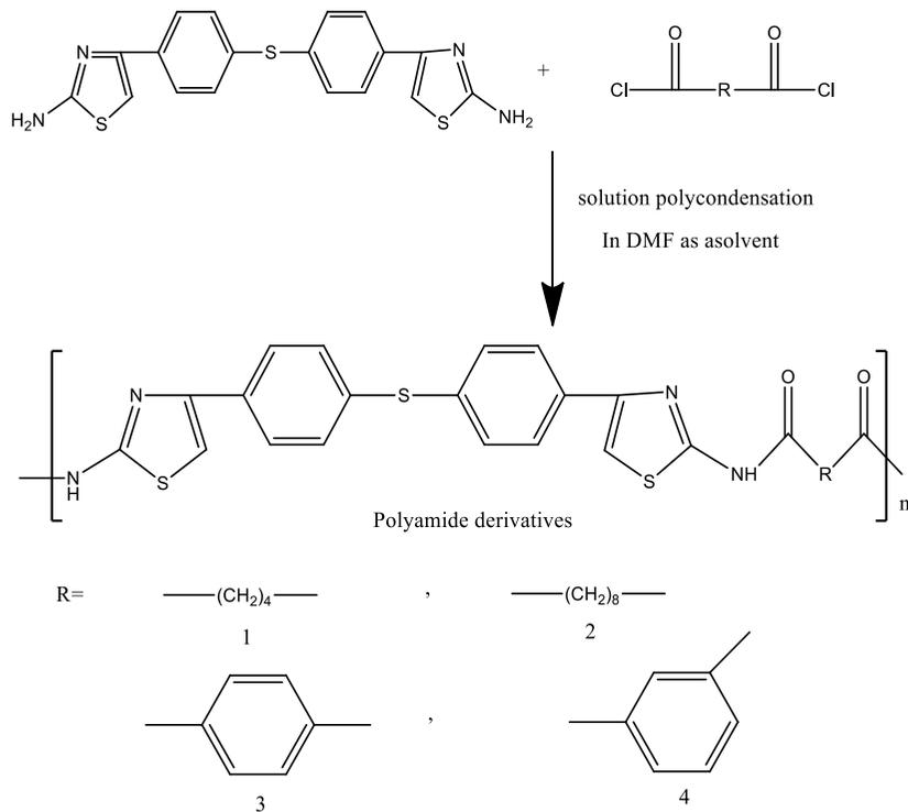
**Figure 2.** Synthesis of the polyamides PA<sub>1-4</sub> derivatives.
