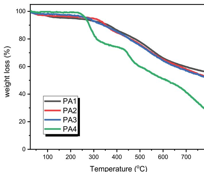
**Figure 4.** TGA curves of PA<sub>1</sub>, PA<sub>2</sub>, PA<sub>3</sub> and PA<sub>4</sub> in air-flow at a heating rate of 10 °C/min.
