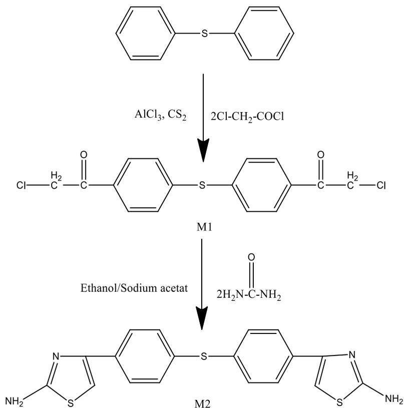
**Figure 1.** Synthesis of bis-4-chloroacetyl-diphenylsulfide M1 and 2-aminothiazole-diphenylsulfide M2 monomers.
