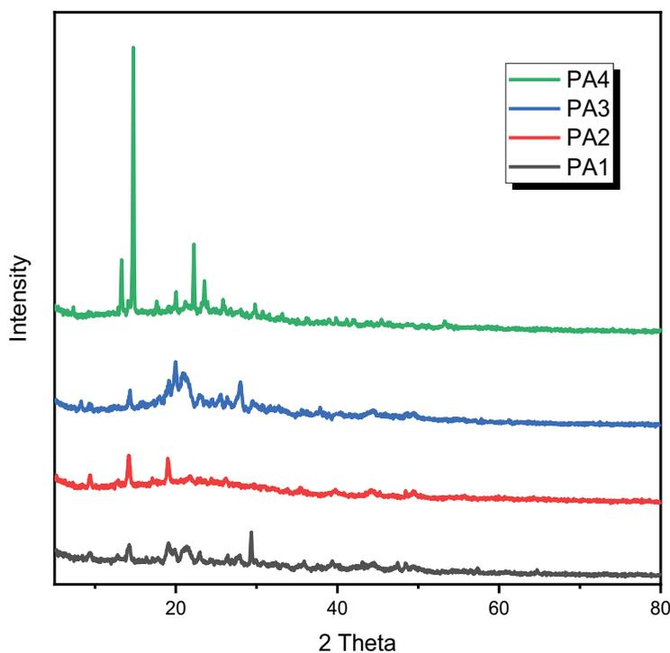
**Figure 5.** XRD of polyamides PA<sub>1–4</sub> derivatives.
