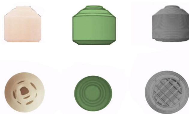
Figure 5. 3D-printed pregabalin gastrofloating tablets. The internal structure of tablet is composed of a grid infill with void space filled with air so that the tablet has low density, which helps the buoyancy of the tablet in media [32].
