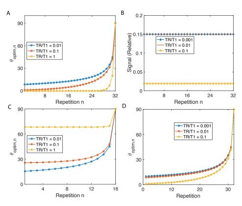
**Figure 2.** Variable flip angles for constant signal and maximum signal. (**A**) The flip angles to enable constant magnetization in a 32 repetition imaging sequence are determined based on Equation (7). (**B**) Implementing flip angles in (**A**), the relative transverse magnetization signal is simulated taking  $K_{\rm hp} = 1$  and  $K_0 = 10^{-3}$ . (**C**,**D**) The flip angles to maximize the cumulative signal under different TR/T1.
