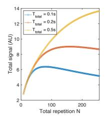
**Figure 7.** Total signal with RARE sequence. The simulation is conducted based on parameters close to diamonds ( $T_1 = 50$  s,  $T_2 = 1$  ms, TE = 0.5 ms). The total signal curve S(N) maximize at different N when  $t_{total}$  is set to different values.
