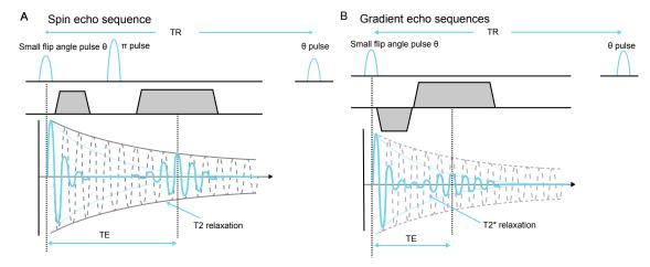
**Figure 4.** Spin echo and gradient echo sequence with small flip angle. (A) The  $\pi$  pulse refocuses dephasing caused by field inhomogeneity, chemical shift, and gradients. (B) The reversed gradient refocuses the effect of gradients. The phase encoding dimension implements same gradient arrangement for both of the two echo sequences, and is omitted here.
