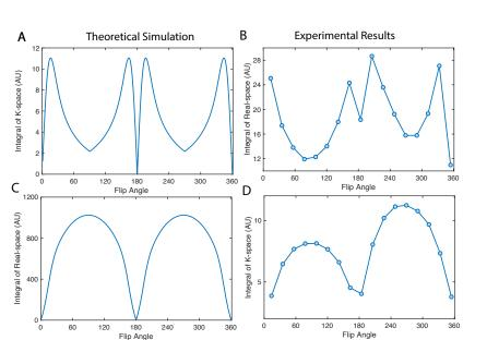
**Figure 6.** Total signal in k- and real- space as a function of flip angle. (**A**,**B**) The integration of absolute value in k-space is simulated and measured using the diamond particle phantom. (**C**,**D**) Display the integration of absolute value in real-space. The simulations are conducted assuming a uniform profile in real-space, i.e.,  $\rho(x, y) = \text{constant}$ , in which case only the effect of magnetization factor *K* is emphasized.
