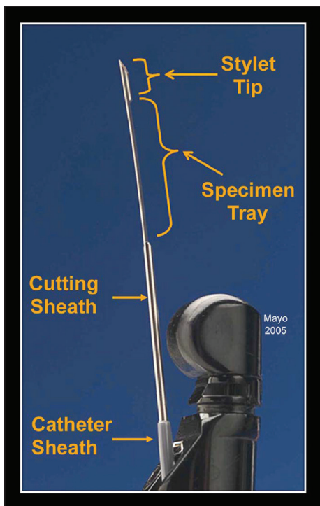
Figure 1. Non-handle portion of the Tru-cut needle demonstrating the following: Outer “catheter sheath,” an internal 19-gauge “cutting sheath” that shaves off the tissue specimen; an 18-mm-long “specimen tray,” which contains the tissue core; and a 5-mm-long “stylet tip.” Adapted with permission from Levy and Wiersema
