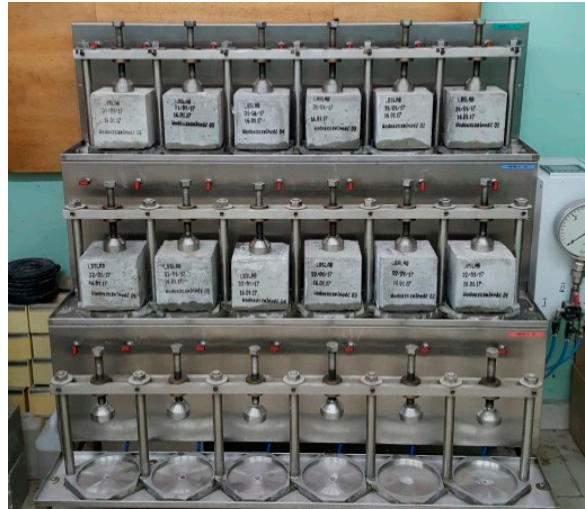
Figure 3. Water-tightness test of concretes.
