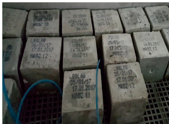
Figure 4. Frost resistance test of concretes.
