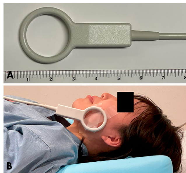
Fig. 1. A. Microscopy coil. B. The microscopy coil is fixed to the skin surface near the left first molars with surgical tape.
