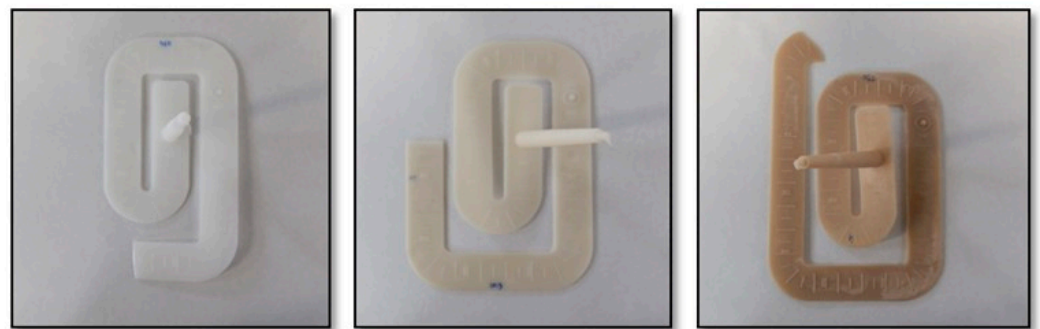
Figure 8. Spiral specimens for PA6 (left) and star polyamides modified with 2.5% (center) and 5% (right) 5-aminophthalic acid.
