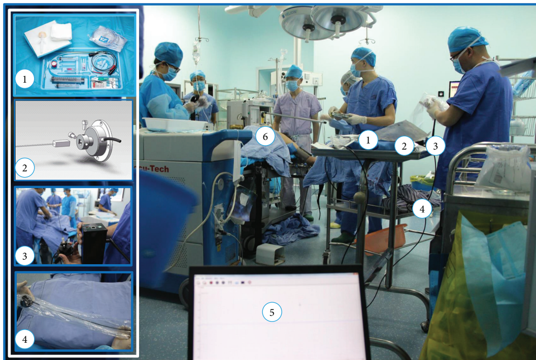
FIGURE 3: Clinical trial setup for the multichannel intraoperative data collection. Component details are as follows: 1: biopsy surgical instrument; 2: force sensor (ATI Nano17) +3D print connector; 3: line puncture device integration; 4: data conversion; 5: analysis software; 6: patient.
