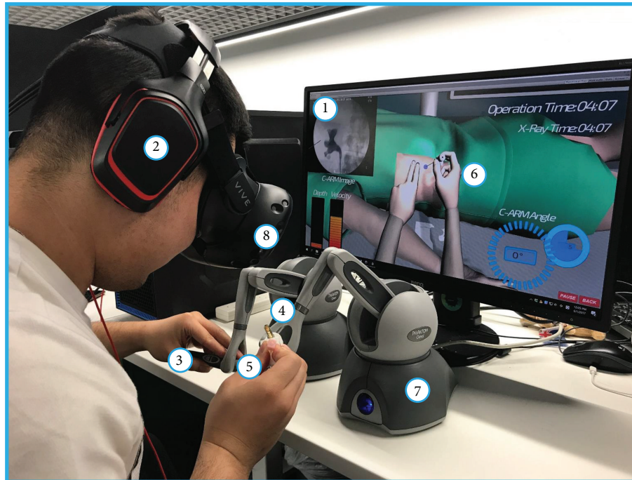
FIGURE 5: The immersive virtual training platform with an i7 6700 (3.4 GHz) CPU workstation, 8 GB memory, and 1070 NVIDIA Graphics GPU. Two PHANTOM Omni reproduce the dual-hand force rendering, HTC VIVE provides the 3D visual rendering with head tracking, and a Beat Solo 2 wireless headphone provides the real-time surgical audio. Component details corresponding with the operation room are demonstrated in Table 2.
