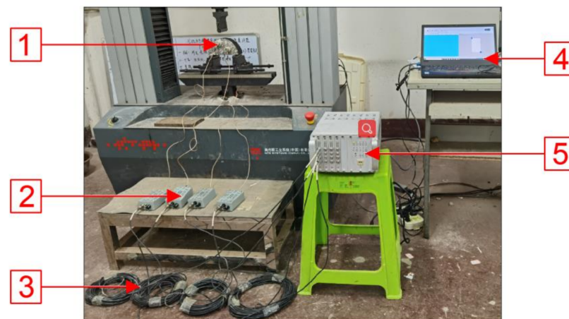
Figure 4. AE test system: 1: G8 sensors; 2: Preamplifier; 3: Cable; 4: Computer; 5: High-speed digital AE detector.
