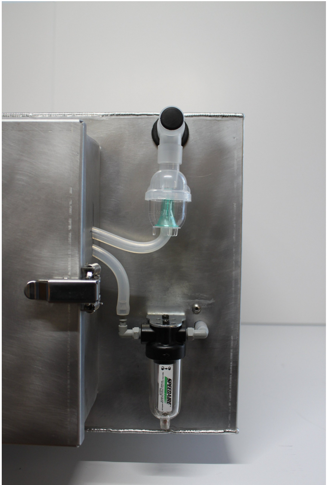
Fig 3. Arca exterior showing nebulizer (top), condenser unit (bottom), and electronics housing (left).
