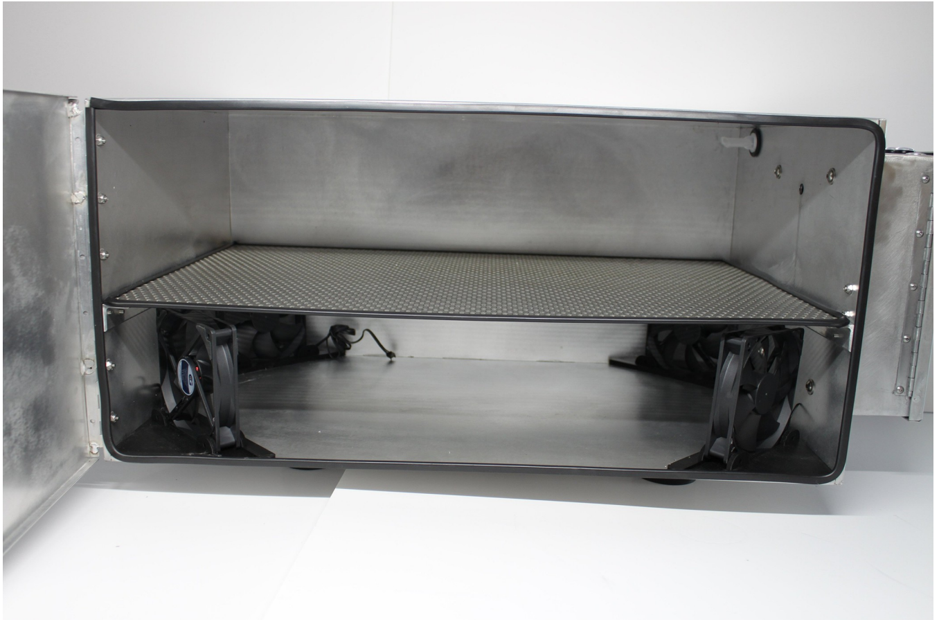
Fig 2. Arca interior demonstrating mesh rack, circulating fans, and Venturi tube nozzle.
