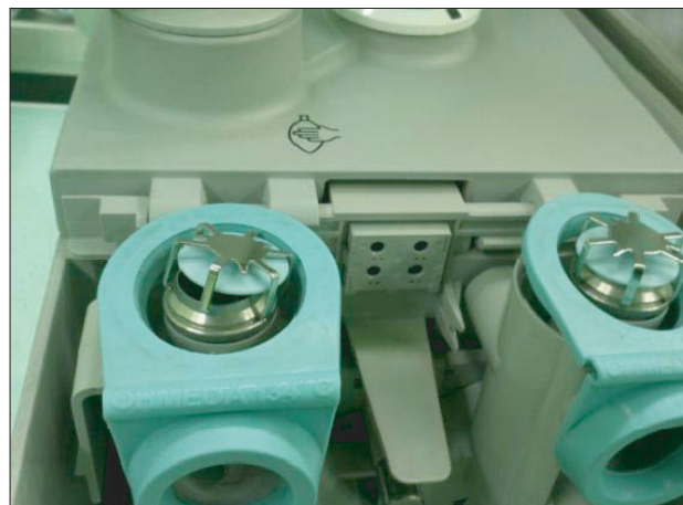
Fig. 4. Properly connected expiratory unidirectional valve (Right) and improper orientation of disk and disc locking apparatus (Left). Note that the disk locking apparatus of which its foot is not put on the groove of valve.
