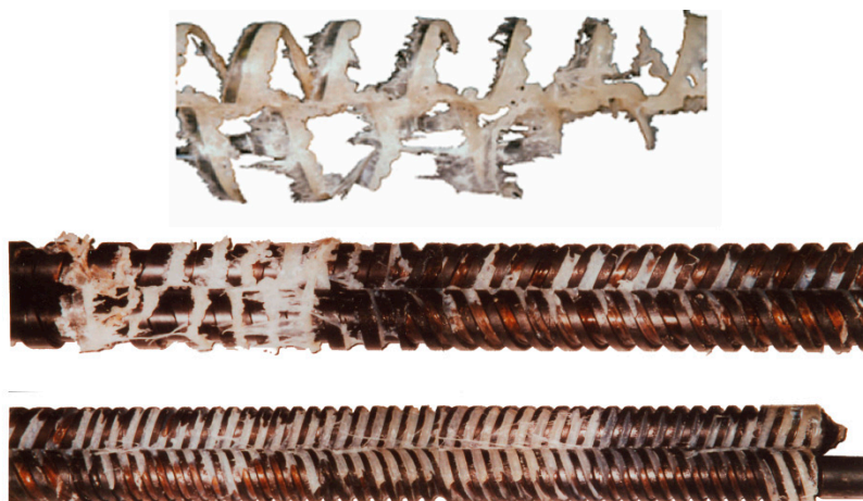
Figure 3. Melting mechanism for counter-rotating twin-screw extrusion [120].
