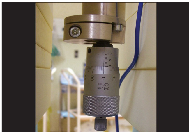
Figure 2: Micrometer design for selection of plate separation in the extrapolation chamber (EC)
