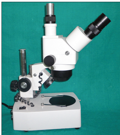
Figure 7: Stereomicroscope used for evaluation of microleakage
