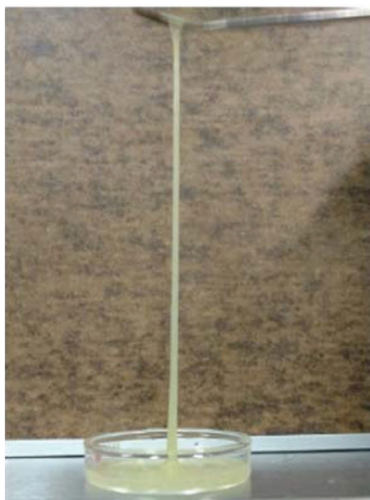
FIGURE 6 Picture of the solution with 6 wt.% of M mucilage subjected to elongation and showing its state of high elasticity
