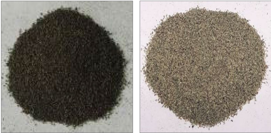
Fig. 2 The biosorbent materials in the final form before application of batch and continuous flow trials. The left one is colored sample, and the right one is the decolored sample
