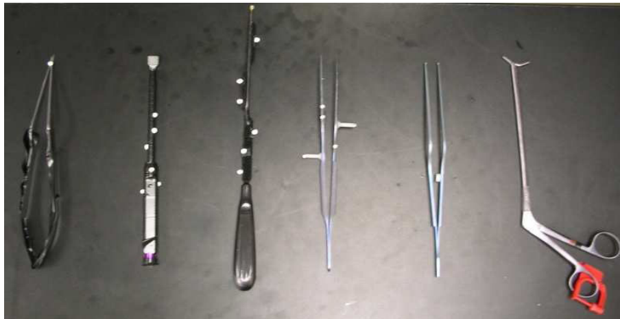
Figure 9 Common surgical tools: reflective markers attached to them for motion tracking purposes, the Rasp is second from left.
