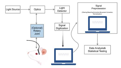
Figure 1. Schematic of the setup of a generic rodent in vivo fiber photometry experiment.
