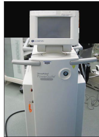
Figure 1: The 100 watt Versapulse holmium laser used to perform HoLEP
