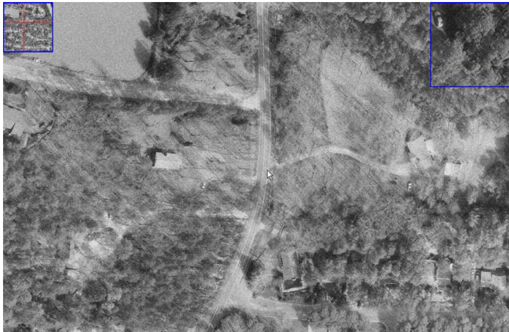
Fig. 1. Sample screen from the Pointer interaction technique. The target is shown on the top right . The navigation overview is on the upper left , with crosshairs showing the current cursor location. The user is currently at Zoom Level 3 and positioned slightly above and left of the center of the full image.
