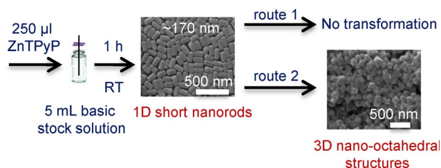
Figure 3. Illustration of the shape transformation from short nanorod structures to nano-octahedral structures.
