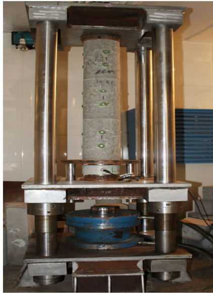
Figure 2. Reaction frame for creep test.
