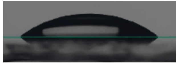
FIGURE 4: Baseline positioning using droplet reflection.
