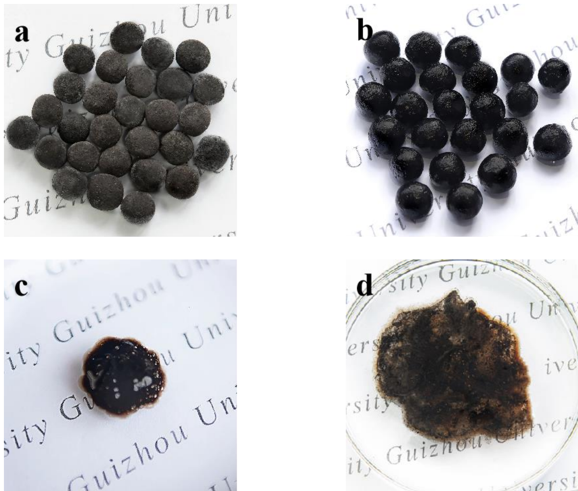
Figure 13. Electronic digital photograph of fertilizer: (a) fertilizer core, (b) ADP@PAA-KHA, (c) ADP@PAA-KHA absorbs water for 20 min, and (d) ADP@PAA-KHA absorbs water for 24 h.
