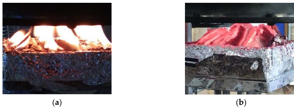
Figure 10. Wood samples coated with the formulation D after a 20 min exposure to a heat flux of: (a) 30 \text{ kW/m}^2 and (b) 50 \text{ kW/m}^2 .
