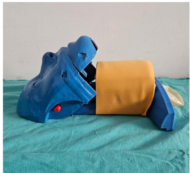
Fig. 3 3D printed manikin with layers for obese simulation
