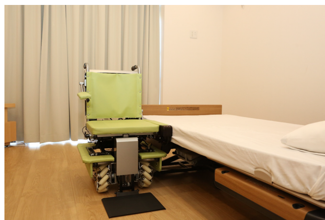
Figure 1 Example of a lateral-transfer type system The lateral-transfer type system has an innovative approach to performing easy transfers: electrically adjustable armrests and seat, easy rotation in any direction, ability to move easily to any location.
