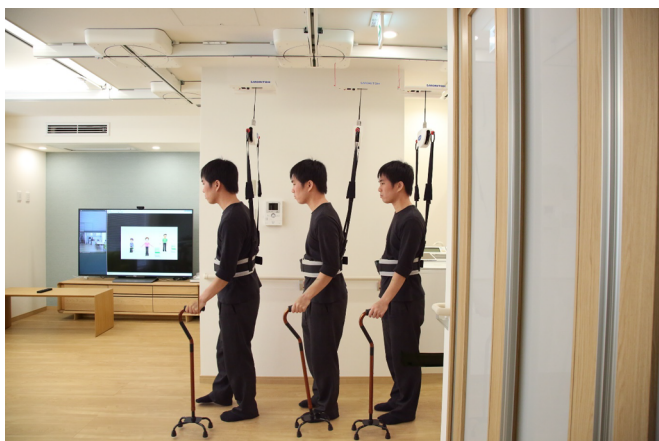
Figure 2 Example of a suspension-type system (walking support robot, Moritoh Co., Ltd.)
