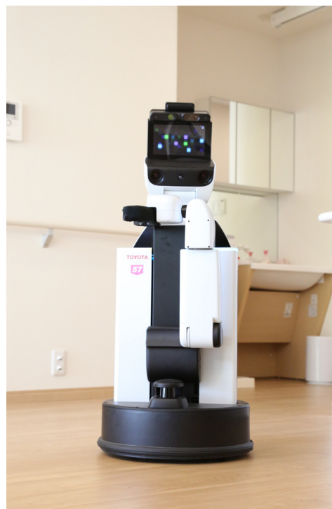
Figure 3 Example of an operational assist system (human support robot, Toyota Motor Corp.)
