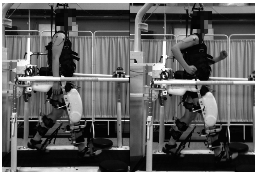
Figure 1. The experimental apparatus and the tasks used. Each subject walked passively in the DGO and kept his lower extremities relaxed throughout the session, with different tasks for the upper extremities. In the first experiment, the subject walked without (left panel) and with (right panel) arm swing. In the second experiment, he walked with the arms swinging while wearing different loads on both wrists.
