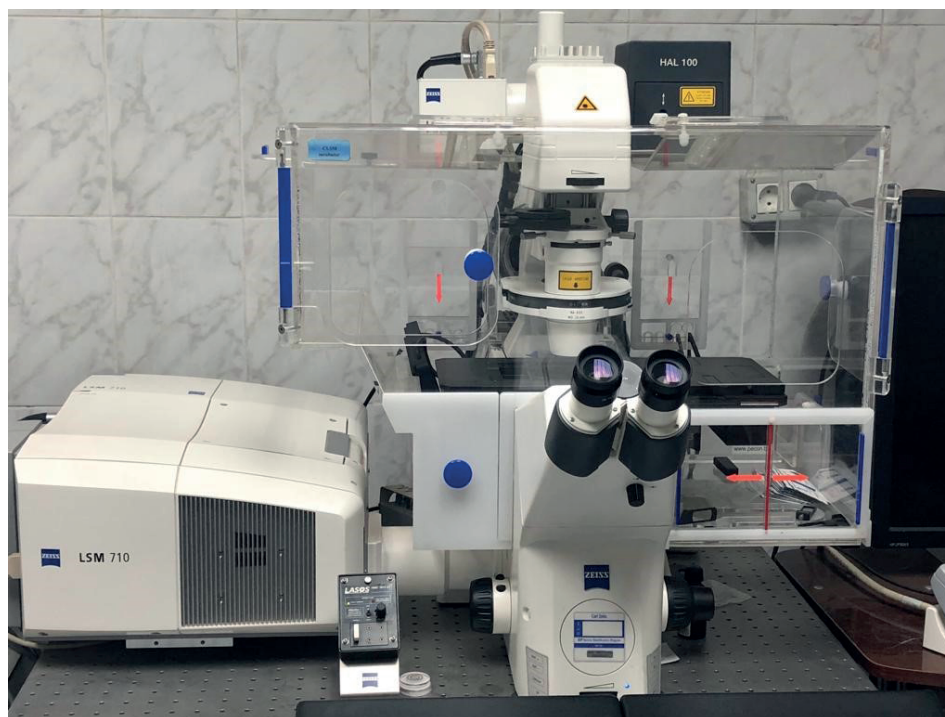
Figure 1. A Zeiss LSM 710 confocal laser scanning microscope.
