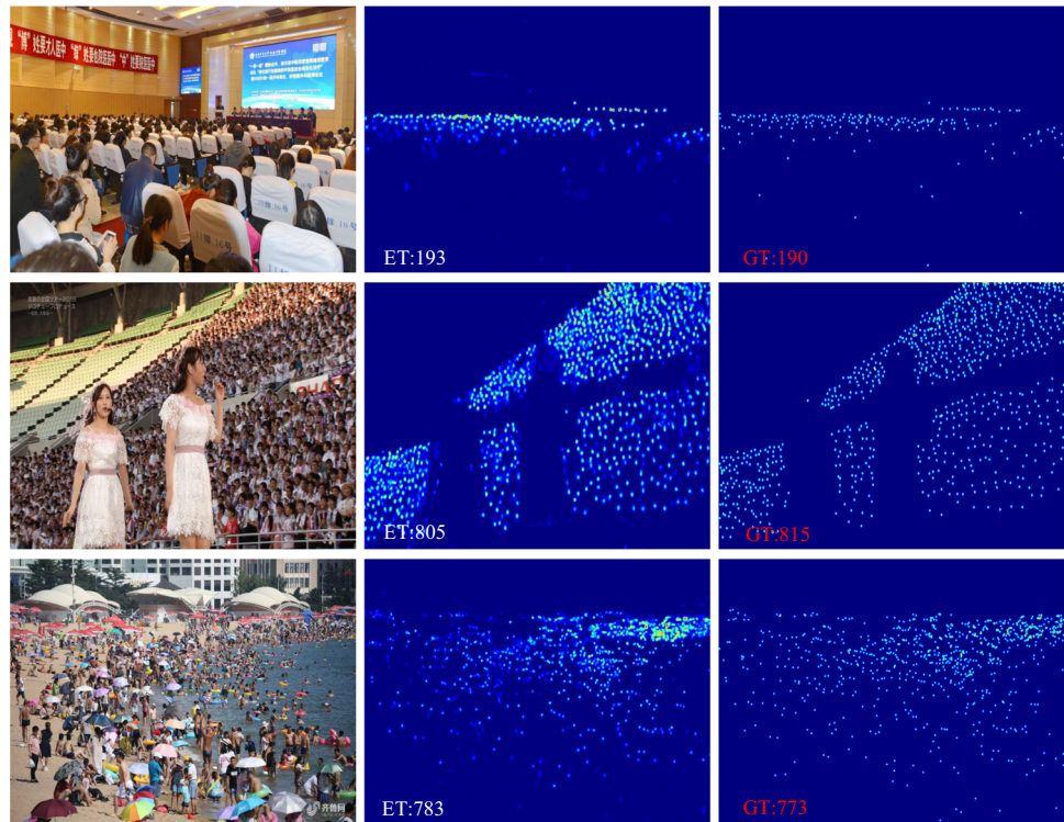
Fig. 10 The exhibition of the ground truth density maps and estimated density maps generated by the proposed DRNet on NWPU-Crowd dataset. The first column denotes input crowd images. The second column and the third column present estimated density maps and ground truth density maps, respectively. GT and ET represent ground truth crowd numbers and estimated crowd numbers
