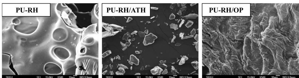
Figure 7. FE-SEM images of the residual chars of PU-RH, PU-RH/ATH 125 , and PU-RH/OP 20 after the cone calorimetry test.
