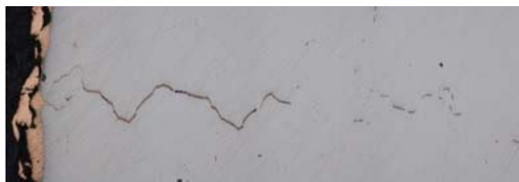
Figure 2. Copper infiltration into a S345J steel matrix.
