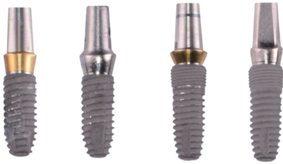
Fig. 1. Implant-abutment assemblies. In order from left to right: Os-P (Osstem TS II implant - Prefabricated TS transfer abutment, Osstem Implant), Os-C (Osstem TS II implant - CAD/CAM customized abutment, Osstem Implant), De-P (Implantium implant - Prefabricated Dual abutment, Dentium), De-C (Implantium implant - CAD/CAM customized abutment, Dentium).
