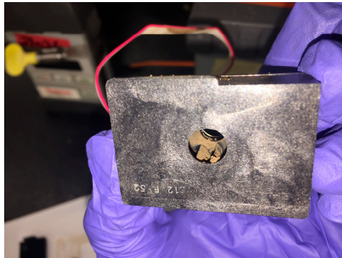
Figure 9. Dust fouled the active Sharp sensor after just 19 weeks of deployment in the factory.
