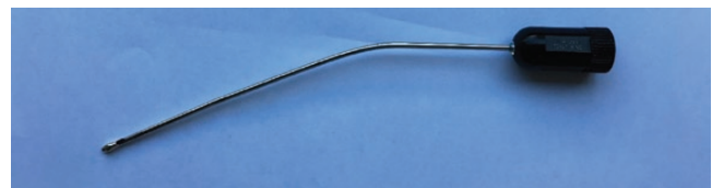
Figure 6. Bended bulb cannula after compression test with RSC-925 at 90°.
