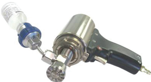
Fig. 18.1 A high-pressure jet injector used to vaccinate pigs. This instrument is powered by either compressed air or liquid CO 2 . It delivers a vaccine dose of 0.1ml to 0.5ml. (Courtesy of Pulse NeedleFree Systems, Inc.)
