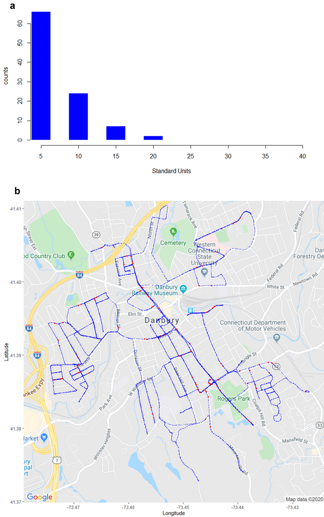
Figure 8. a: Histogram of z-scores for Predicted Leaks in Danbury, 2019. b: 2019 Danbury Survey Results Map (blue = measurement, red = leak).
