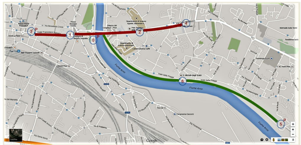
Figure 1. Fixed sensor nodes along the Arno River green park (green route) and along a crowded traffic zone (red route). Five nodes were positioned on the red route (nodes 0, 1, 2, 3, and 4). Node 0 was also on the green route, where two additional nodes were positioned (nodes 5–6).
