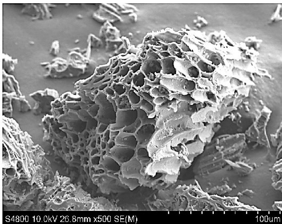
Figure 7. SEM image of highly porous characteristics of activated carbon full of cavities. Adapted with permission from Ref. [107].
