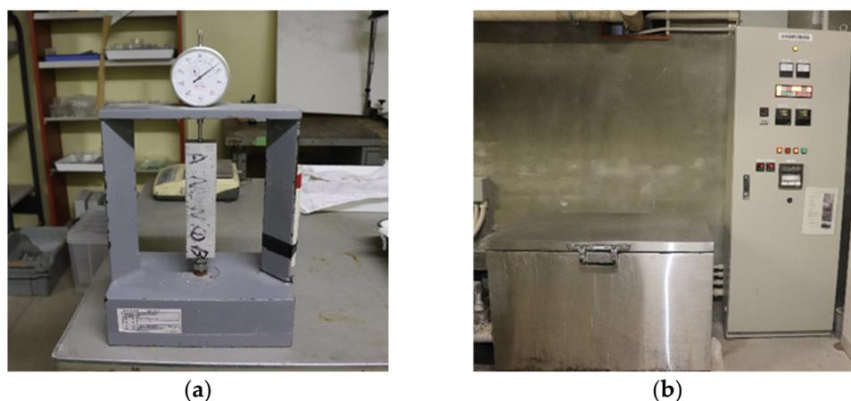
**Figure 2.** Photographs of the test equipment: (a) dial gauge used to measure length-change ratio of dry shrinkage test; (b) the test tank of freeze–thaw test.
