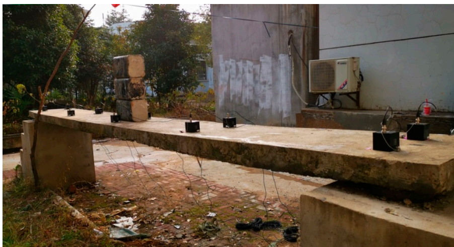
Figure 12. The simply supported reinforced concrete plate with additional mass blocks.
