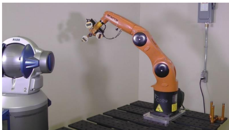
Figure 8. Validation of the robot accuracy in 500 joint sets with a FARO laser tracker.
