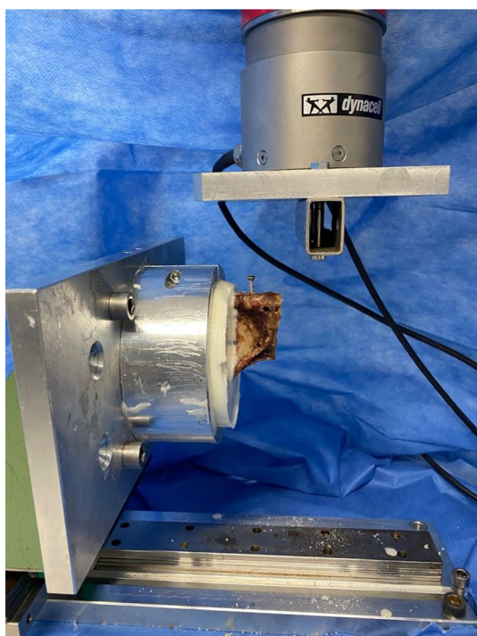
Fig. 2 Experimental setup prior to pull-out (linear slide used to eliminate shear forces and to position specimen)
