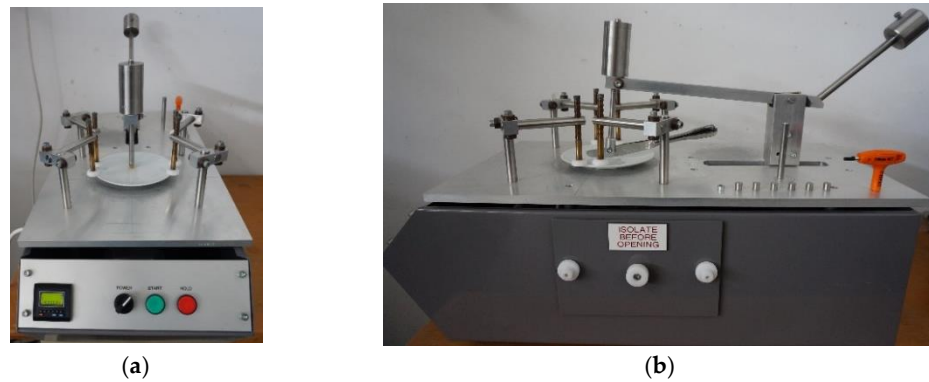
Figure 11. Metal marking machine (a) front view with steel ball test; (b) side view with a knife fixed to the moving arm. Manufacturer: Anderen Limited, Stoke-on-trent, UK.
