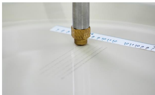
Figure 15. CTCV metal marking test on a porcelain dish.
