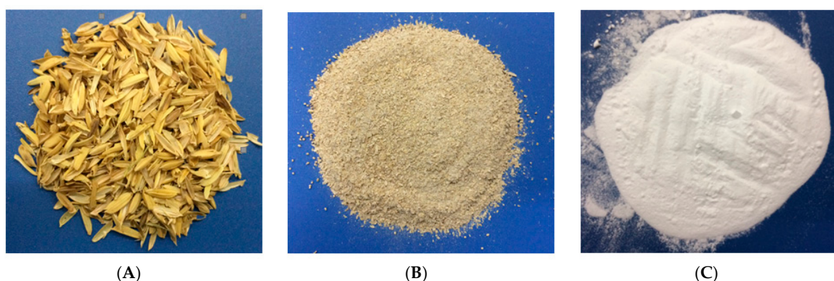
Figure 2. Pictures of (A) rice husk; (B) milled rice husk; and (C) synthesized nanosilica.
