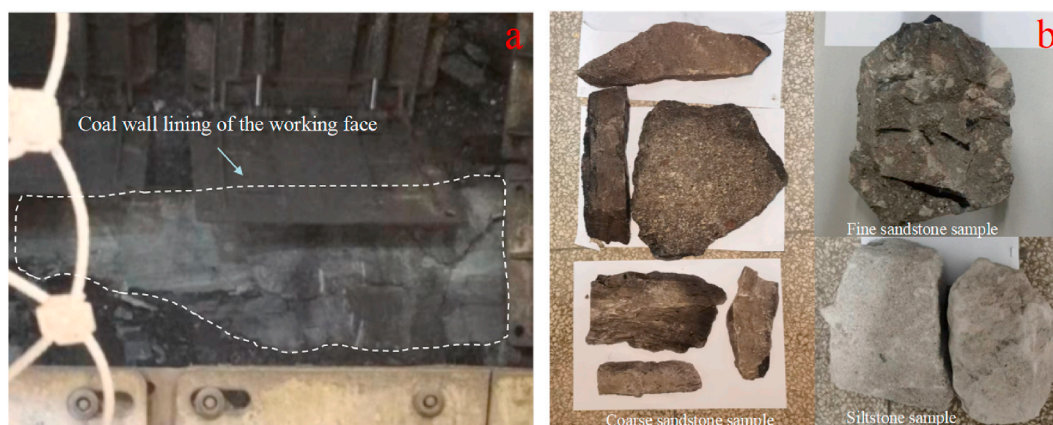
Fig. 1. Experimental samples (a is empirical evidence of sandstone rock exposed in the coal wall of the working face, b is partial sandstone sampling).
