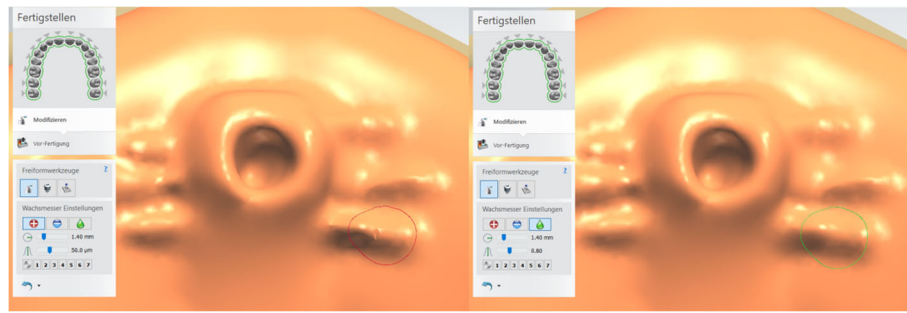
Fig. 4 Design of the stimulation element in freeform (left). Smoothing tool to remove sharp edges (right)
