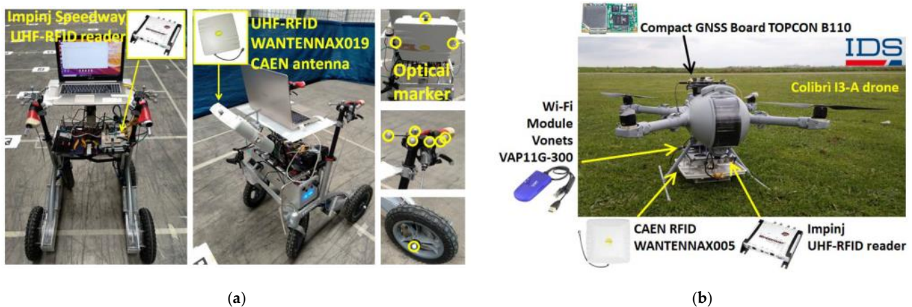
Figure 15. (a) Robotic wheeled walker equipped with the Impinj Speedway Revolution R420 UHF-RFID reader, the reader antenna, and optical markers used for the measurement campaign in [120], © 2021 IEEE; (b) Colibri I3-A drone by IDS, equipped with a GNSS module and the UHF-RFID reader and antenna used in [122], © 2019 IEEE.
