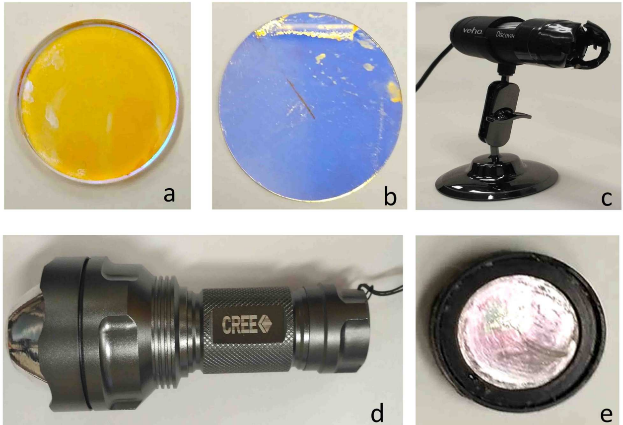
Fig 2. Components of the proposed microscope: (a) Dichroic mirror (b) Exciter filter (c) Pocket microscope (d) Flashlight (e) Barrier Filter.
